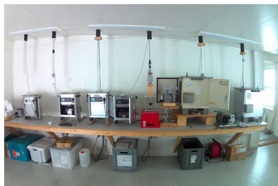
Aerosol sampling devices operated at Gruvebadet observatory since 2010 by University of Florence in close cooperation with CNR-ISP. (Photo: Mauro Mazzola)
