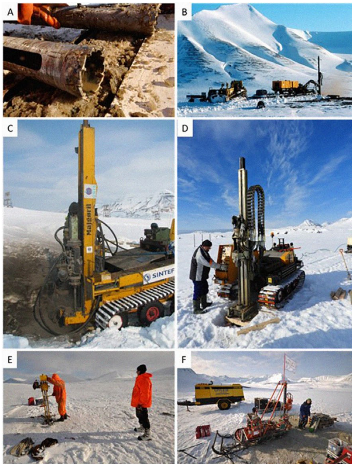
Figure 3: A) Single core barrel. Squared tungsten carbide inserts form the crown of the drill bit. (Photo: Ullrich Neumann). B) Borehole being drilled in Janssonhaugen. Drill rig, air compressor and accessories are placed onto one large sledge (Photo: Johan Ludvig Sollid). C) Rotary percussion drilling at Endalen borehole with the Geotech 504 geotechnical drill rig. (Photo: Håvard Juliussen). D) The Hornsund GM 50 GT Combi drill rig. (Photo: Tomasz Wawrzyniak). E) Russian drill rig in operation near Barentsburg. (Photo: Ullrich Neumann) F) UNIS permafrost drill rig drilling the DBNyÅlesund borehole. Kings Bay AS supplied the air compressor (Photo: Ullrich Neumann).
