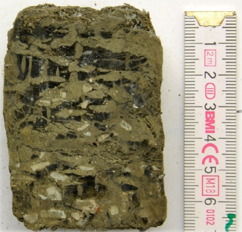
Ice-rich permafrost at 150 cm depth from the Endalen borehole site. The darkest parts are ice lenses, while the rest are cobbles and sediment. (Photo: Ullrich Neumann)
