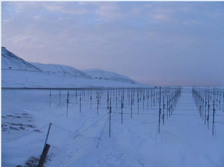
Antenna array – 356 Yagis - improvement #1
