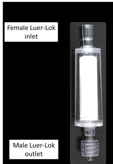
Fig. 7.15-1 Left: Sterivex filter with indication of inlet and outlet; Right: Peristaltic pump filtration set-up
