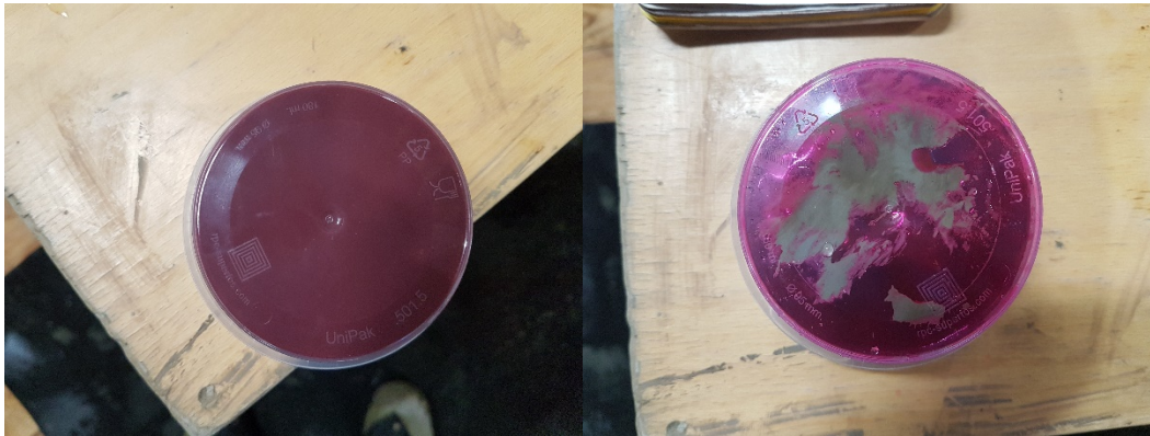
Fig. 15.1.1.1-1 Well-mixed sample (left) and not sufficiently mixed sample (right).
