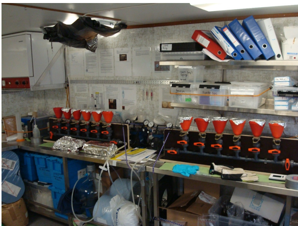
Fig. 1 Example of a filtration set-up.
